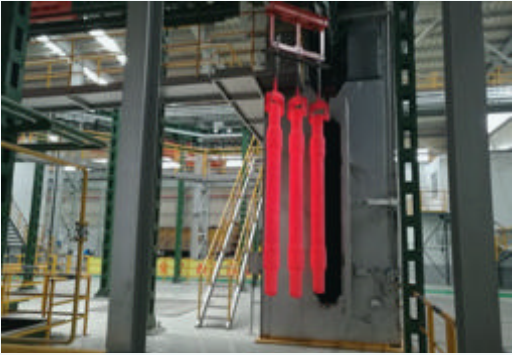
© The axle forging production line can realize the automatic transmission and data acquisition of the whole process of axle from billet heating, forging, straightening and slow cooling
